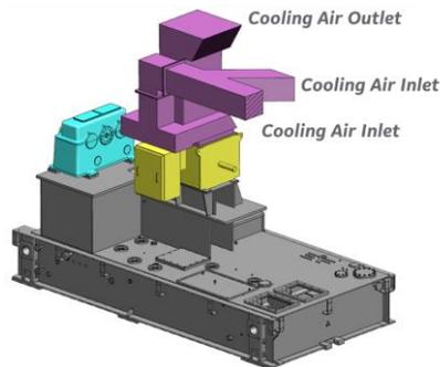
Figure 7 EM air cooling system
