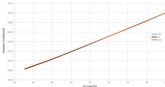
Figure 11 GT emissions vs power output
