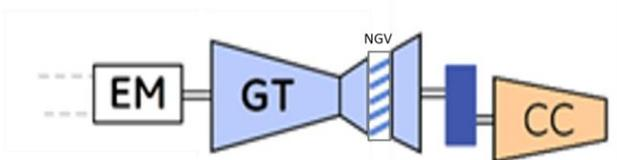
Figure 6 HP shaft hybrid configuration
